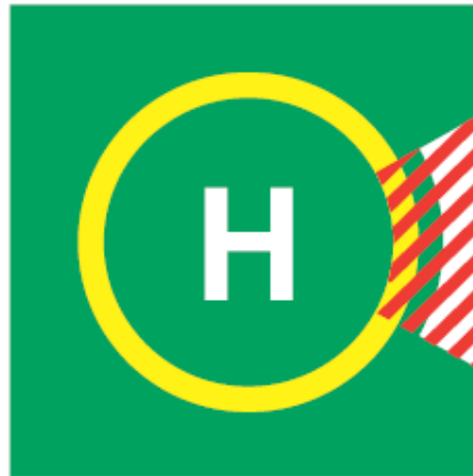
Figure 5-5. Helideck prohibited landing sector marking
