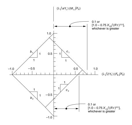
Figure P-3A—Construction of Nomogram for b<sub>1</sub>, b<sub>2</sub>, c<sub>1</sub>, c<sub>2</sub> Boundary
