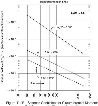
Reinforcement on Shell (L / 2a = 1.5)
