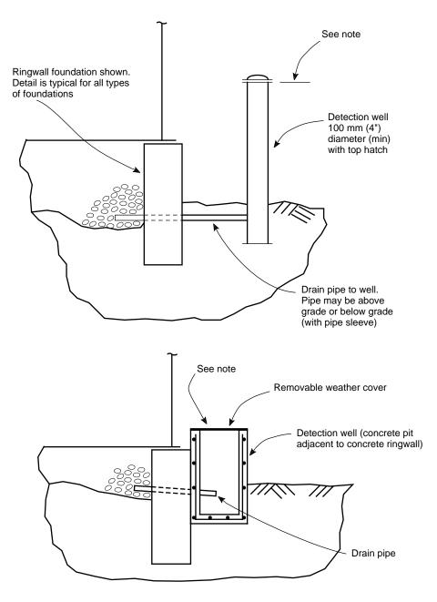
Note: Top of well shall be above maximum high water level within dike.
