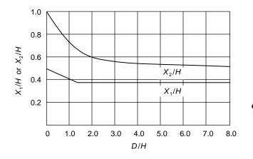
Figure E-3—Centroids of Seismic Forces
