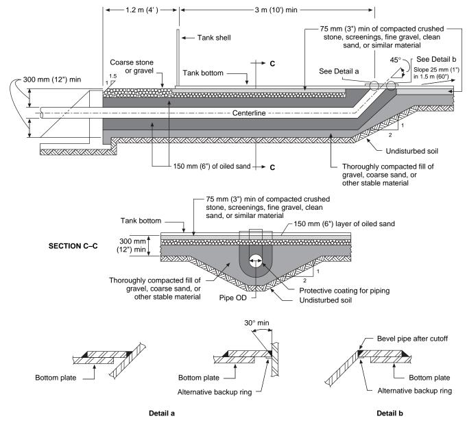
Note: This type of connection shall not be used for tanks with a diameter of less than 6 m (20 ft).
