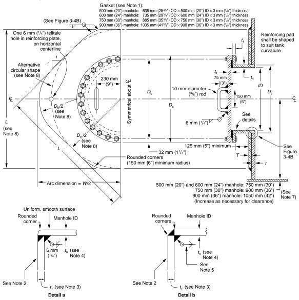
500 mm (20") and 600 mm (24") shell manholes: twenty-eight 20 mm-diameter ( $^{3}/_{4}$ ") bolts in 24 mm ( $^{7}/_{8}$ ") holes 750 mm (30") and 900 mm (36") shell manholes: forty-two 20 mm-diameter ( $^{3}/_{4}$ ") bolts in 24 mm ( $^{7}/_{8}$ ") holes (Bolt holes shall straddle the flange vertical centerline.)
