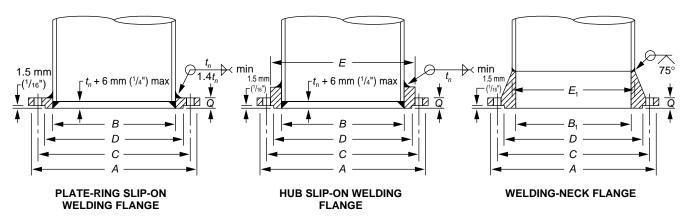
Note: The  $t_n$  designated for weld thickness is the nominal pipe wall thickness (see Tables 3-6 and 3-7).
