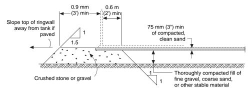
Note: Any unsuitable material shall be removed and replaced with suitable fill; the fill shall then be thoroughly compacted.
