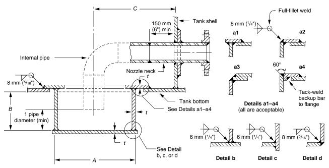
Note: The erection procedure shall include the following steps: (a) a hole shall be cut in the bottom plate or a sump shall be placed in the foundation before bottom placement; (b) a neat excavation shall be made to conform to the shape of the drawoff sump, the sump shall be put in place, and the foundation shall be compacted around the sump after placement; and (c) the sump shall be welded to the bottom.
