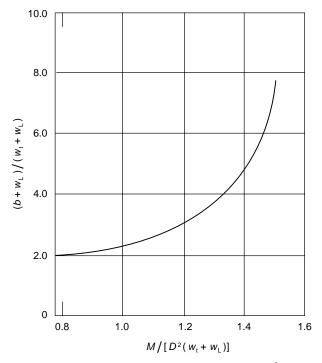
Note: This figure may be used to compute *b* when  $M / [D^2(w_t + w_L)]$  is greater than 0.785 but less than or equal to 1.5 (see E.5.1).
