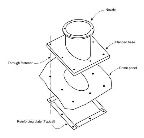
Figure G-2—Typical Roof Nozzle
