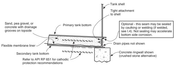
Figure I-4—Double Steel Bottom with Leak Detection at the Tank Perimeter (Typical Arrangement)
