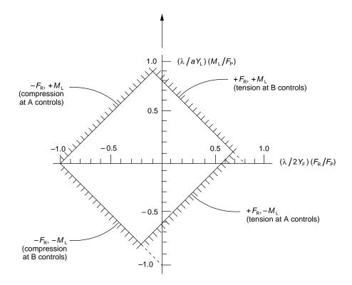
Figure P-5A—Determination of Allowable Loads from Nomogram: F<sub>R</sub> and M<sub>L</sub>
