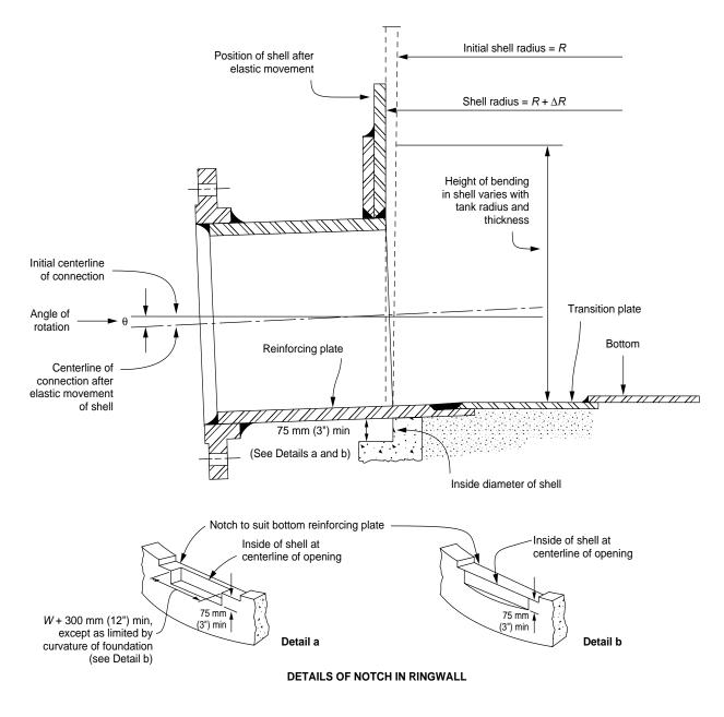
Figure 3-12—Rotation of Shell Connection
