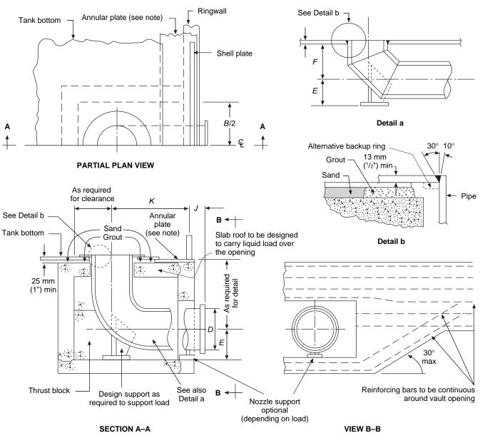
Note: If sketch plates are used, a full plate shall be located over the vault.
