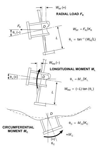
Figure P-1—Nomenclature for Piping Loads and Deformation
