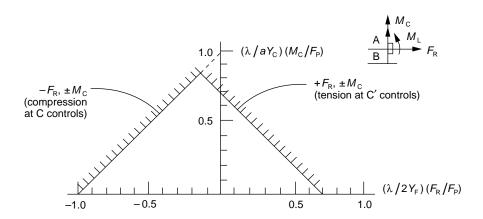
Figure P-5B—Determination of Allowable Loads from Nomogram: F<sub>R</sub> and M<sub>C</sub>
