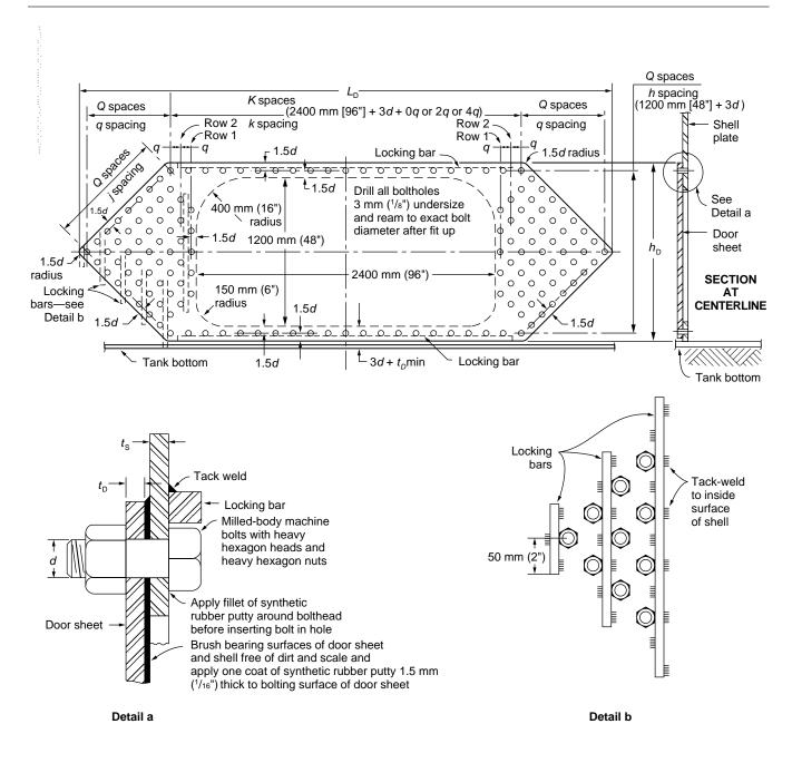
Figure A-3—Raised-Type Bolted Door Sheet (See Table A-6)
