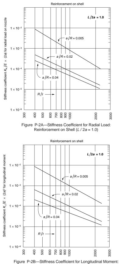
Reinforcement on Shell (L/2a = 1.0)
