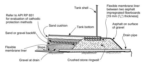
Figure I-2—Crushed Stone Ringwall with Undertank Leak Detection at the Tank Perimeter (Typical Arrangement)
