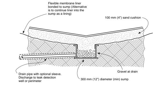
Figure I-9—Center Sump for Downward-Sloped Bottom
