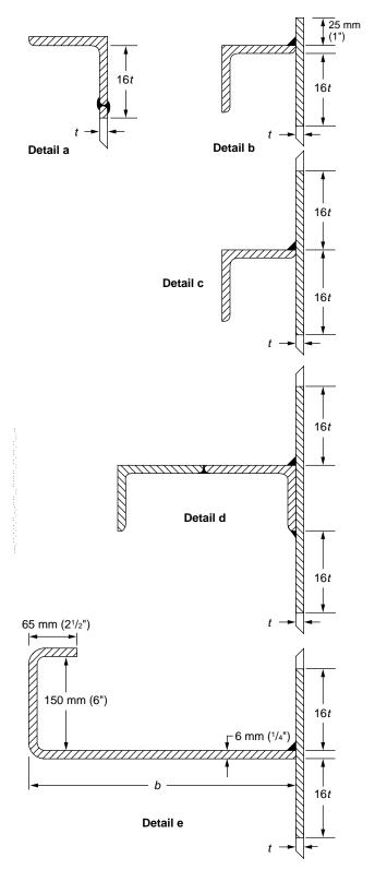
Note: The section moduli given in Table 3-20 for Details c and d are based on the longer leg being located horizontally (perpendicular to the shell) when angles with uneven legs are used.
