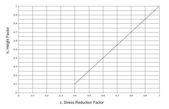
Figure P-11—Stress Reduction Factor
