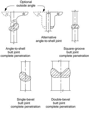
Note: See 3.1.5.3 for specific requirements for horizontal shell joints.
