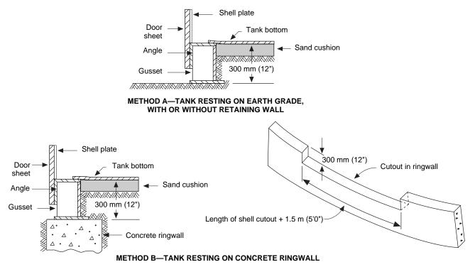
Note: Before the bottom plate is attached to the angle, (a) a sand cushion shall be placed flush with the top of the angle, and (b) the earth fill and sand cushion shall be thoroughly compacted.
